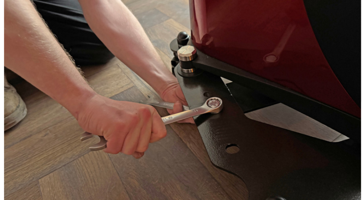
3. Take the 19 mm wrenches and loosen the bolts on the left side of the cart.
